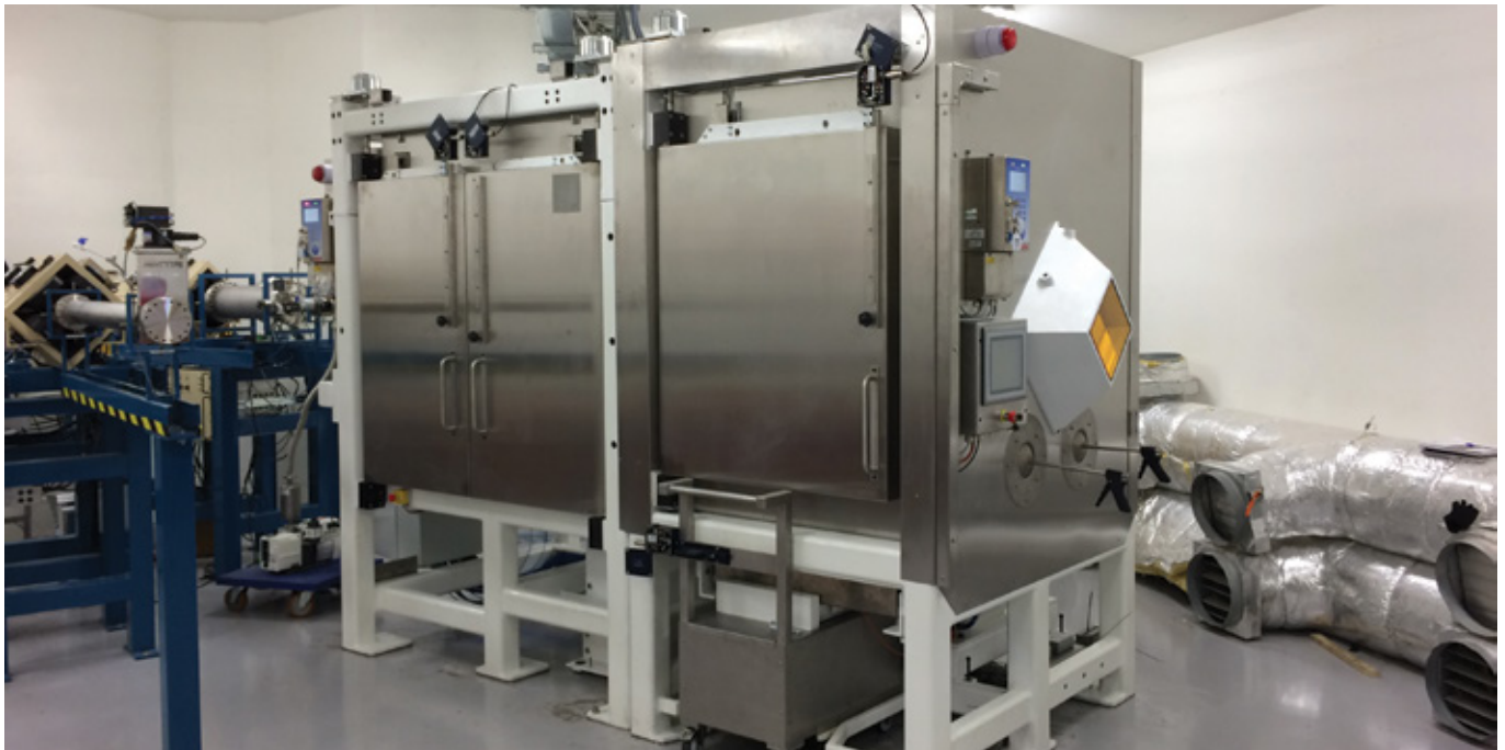
FIG 2. DALTON END OF BEAMLINE PELLETRON ACCELERATOR TARGET HANDLING AND STORAGE HOT CELLS
