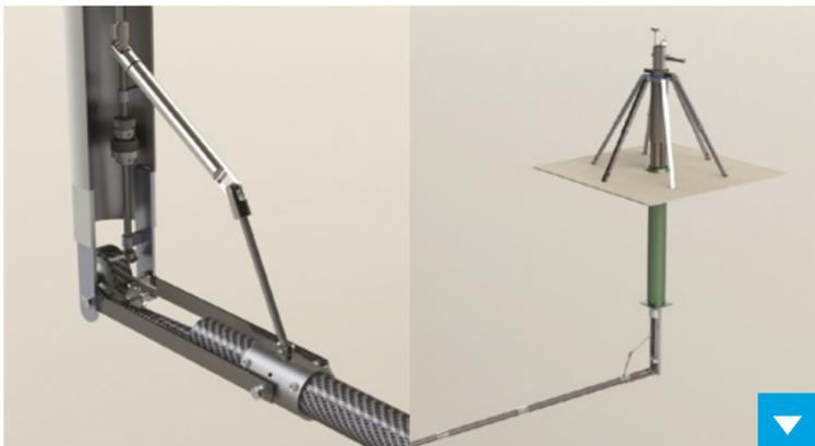
CLOSEUP OF HORIZONTAL ARM AND DRIVE MECHANISMS. FULLY DEPLOYED MECHANICAL ARM WITH HORIZONTAL SECTION PAYED OUT 3M.
