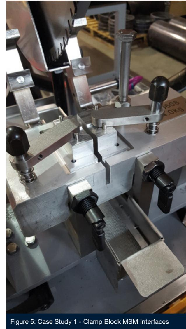
Figure 5: Case Study 1 - Clamp Block MSM Interfaces
