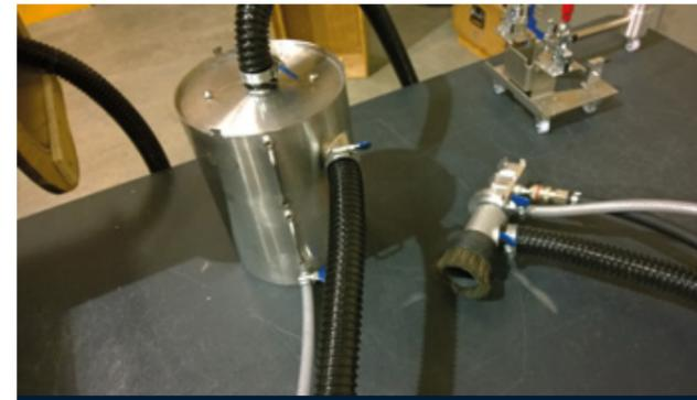
Figure 22: Case Study 3 - Vacuum Blasting Nozzle and Blast Pot
