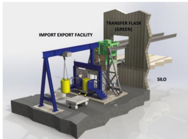
Figure 8: Case Study 2 - Silo, Transfer Flask and Import Export Facility
