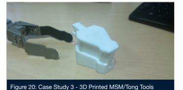
Low cost, standard handles for MSM and tongs, allowing GE
