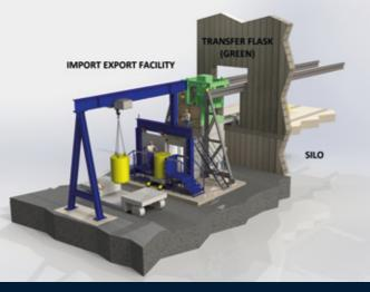
Figure 8: Case Study 2 - Silo, Transfer Flask and Import Export Facility
