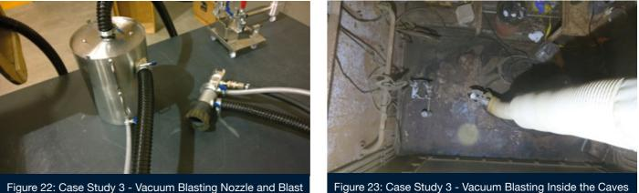
Figure 22: Case Study 3 - Vacuum Blasting Nozzle and Blast Pot
