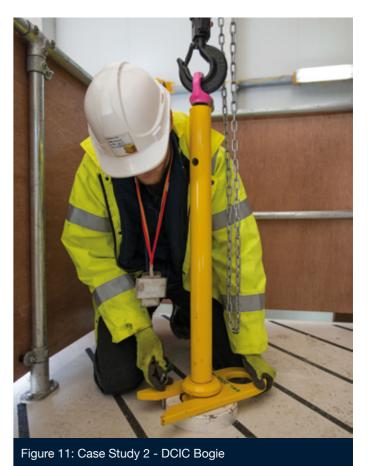
The lid (weighing around 3,000kg) was hoisted up using a suitably rated manual chain hoist and a very basic locking plate fitted around the lid lifting feature so there was no suspended load. Again, the use of COTS equipment here helped to confirm that the operation and design were fit for purpose.
