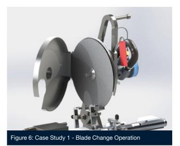
Changing blades between cuts required opening the guard, inserting a gravity engaged pin to lock the motor shaft, and unscrewing a retaining nut on the spindle.
