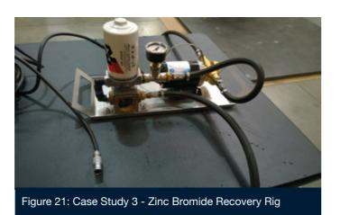
A miniature filtration and pump rig to circulate and filter Zinc Bromide as it is decontaminated through precipitation and ion exchange.
