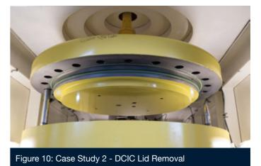
Once the DCIC is inside the shielded cell, the lid is removed by lowering an extension bar through a hole in the roof and screwing it into the lid. This is subject to some 'feel' on the operator's part to know when it is fully engaged, but it is made positive by design and cameras provided for visual confirmation.
