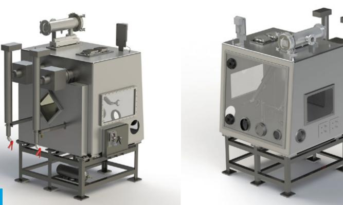
AQUILA MULTI-FUNCTIONAL CELL USED FOR INACTIVE REMOTE HANDLING TRIALS
