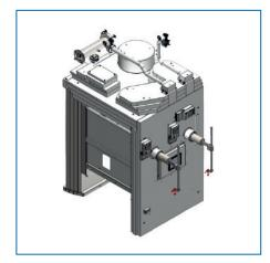
Viewing provision within Hot Cell 1 is provided by a flat screen monitor, coupled to an in-cell camera, mounted on the window aperture blanks. The window blanks offer the ability to replace camera monitoring for a leaded glass window in the future.
