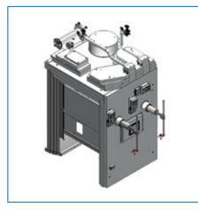
Viewing provision within Hot Cell 1 is provided by a flat screen monitor, coupled to an in-cell camera, mounted on the window aperture blanks. The window blanks offer the ability to replace camera monitoring for a leaded glass window in the future.
