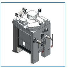
Viewing provision within Hot Cell 3 is provided by a flat screen monitor, coupled to an in-cell camera, mounted on the window aperture blanks. The window blanks offer the ability to replace camera monitoring for a leaded glass window in the future.
