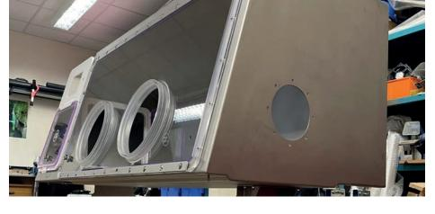
HEPA filter system which allowed their technicians to replace the filter and 'bag out' the used filter without breaking containment.
